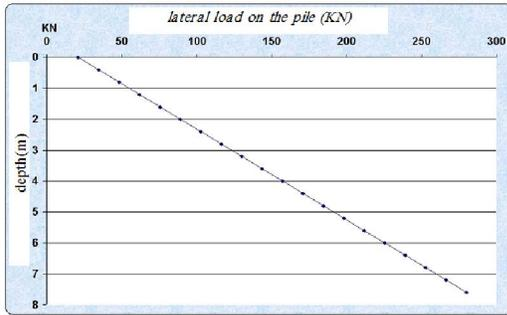
Fig 18- lateral load on the pile with soil 1 by using of Ito & Matsui (1975) equation
