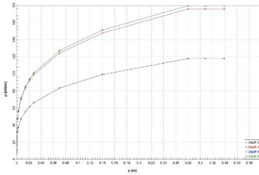
Figure 13- P-Y curve for pile under lateral load
