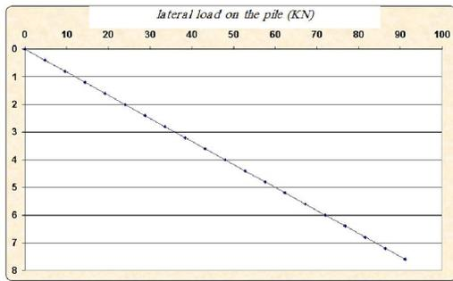
Fig 19- lateral load on the pile with soil 2 by using of Ito & Matsui (1975) equation
